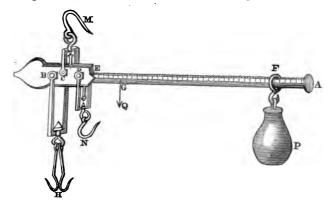
To the point B are attached two hooks H, (or sometimes only one hook or a scale-pan is attached to B), from which the body to be weighed is suspended.
